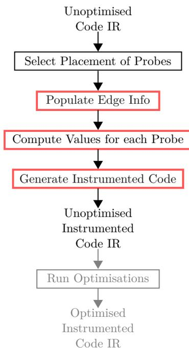
Figure 5.1: Overview of the work instrumentation algorithm.
