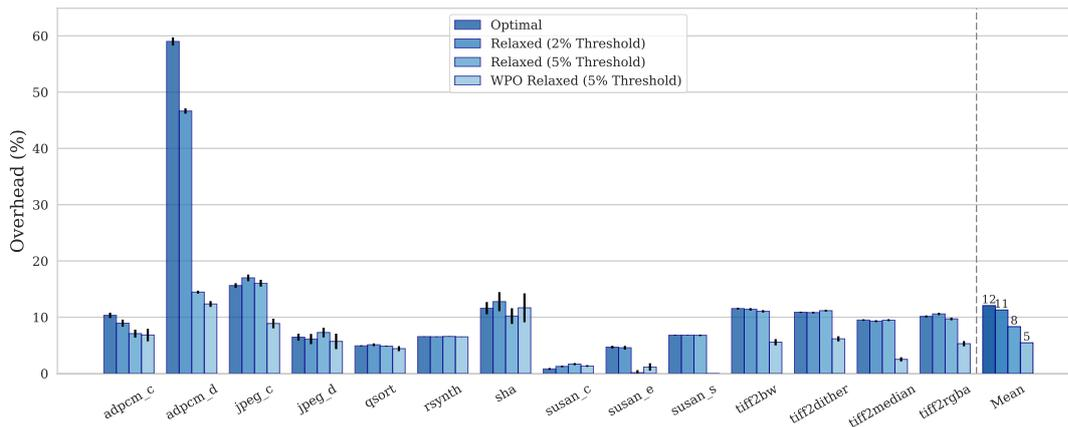
Figure 6.7: Overhead of the instrumentations compiled with `-O3`.
