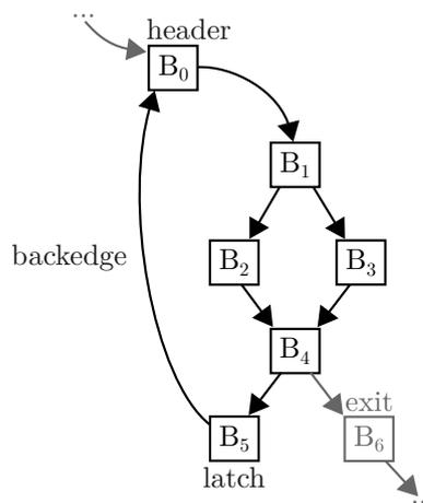
Figure 2.3: Example of a natural loop.
