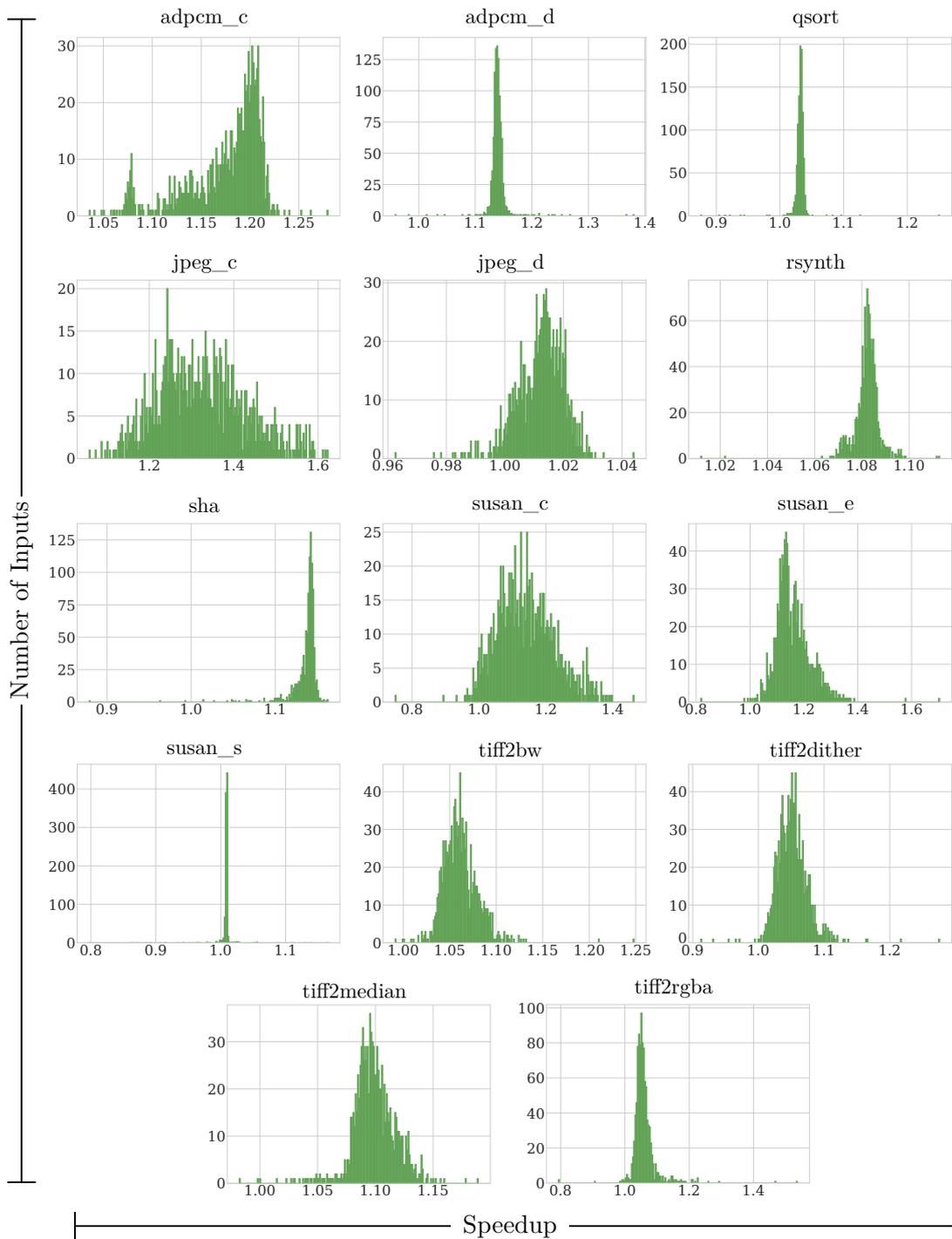
Figure 6.16: Histograms for the speedups over  $-O3$  with the complete dataset of 1000 inputs for each benchmark. In each case, we are using the optimisation sequence with the best average speedup over  $-O3$ . This figure shows how the performance for some of the benchmarks are highly sensitive to the input.
