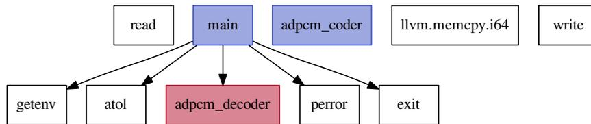
Figure 6.10: Call graph highlighting the maximum basic block frequency of each function, using a cool/warm colour map.
