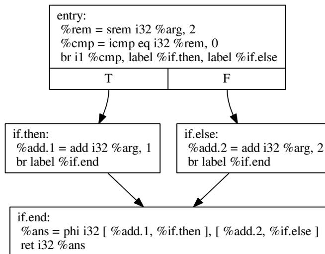
Figure 2.2: Control flow graph of the `odd_inc` function (see Listing 2.2).
