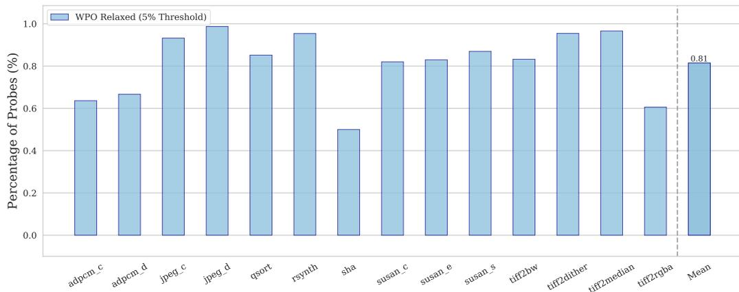
Figure 6.5: Percentage of instrumented basic blocks, after applying a whole program relaxation, relative only to the probes from the optimal profiling that are executed, based on a randomly selected input. In other words, it ignores the probes in basic blocks that were never executed.
